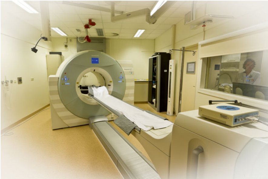
Fig. 3.4 Hybrid camera system, combining positron emission tomography with conventional computed tomography (PET/CT). These camera systems are at present the state of the art, as well. In sports medicine, they can be used for fluorine-18 ( ^{18}\text{F} )-labelled fluorodeoxyglucose PET and ^{18}\text{F} sodium fluoride PET (Image courtesy: Jan Pruim)
