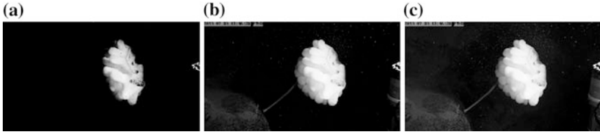
Fig. 13.4 Gray-level transformation of the sponge image. a contrast = 28.0047. b contrast = 40.0722. c contrast = 39.4223
