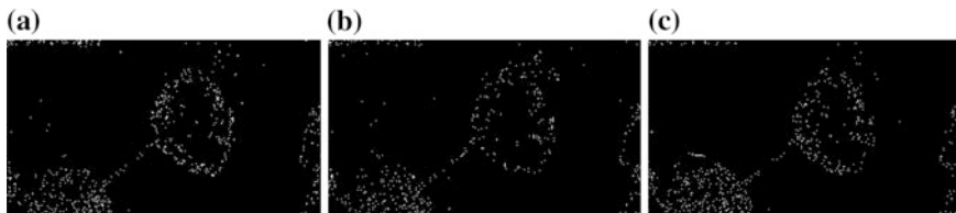
Fig. 13.7 Edge extraction with Prewitt operator, Log operator, and Canny operator. a Prewitt. b Log. c Canny
