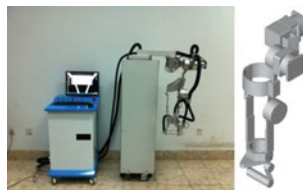
Fig. 6.1 The training system of the five-DOF exoskeleton robot for upper limb rehabilitation
