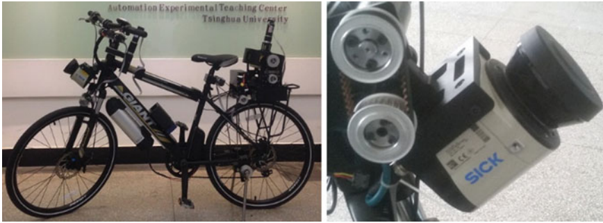
Fig. 22.2 The implemented autonomous bicycle ( left ) and the LRS rotation mechanism ( right )
