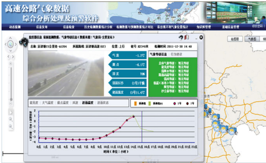
Fig. 31.4 The interface of the comprehensive analysis and early warning expressway weather information system
