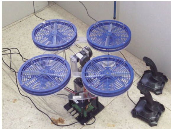
Fig. 51.2 Three-degree-of-freedom quad-rotor hover plant
