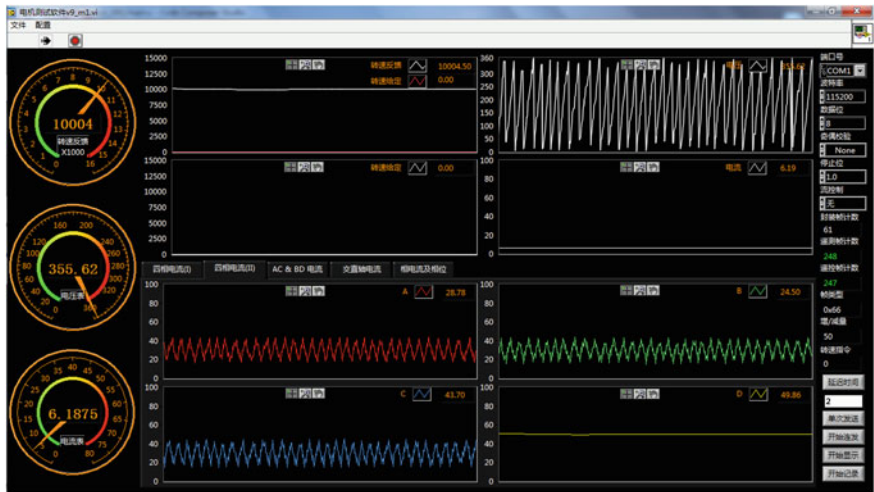
Fig. 52.8 The actual running state of the PMSM with the given speed 10,000 RPM
