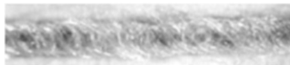
Fig. 4.32 OE friction-spun thread with filament core, 150 tex fineness, CF filament yarn (T300, 67 tex) core, wound about with PEEK fibers (83 tex)
