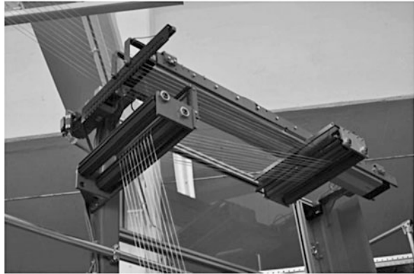
Fig. 7.15 Compensation device for weft yarns (picture shows a yarn tensioning device of the Karl Mayer Malitronic® Multiaxial stitch-bonding machine)
