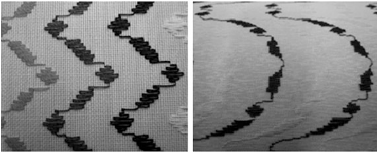
Fig. 5.33 Examples of open reed woven fabric for curtains ( Source: Lindauer Dornier GmbH )
