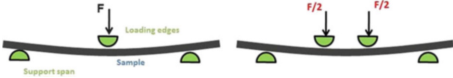
Fig. 14.18 Schematic of a flexural test arrangement according to DIN EN ISO 14125; (a) three-point flexural test, (b) four-point flexural test
