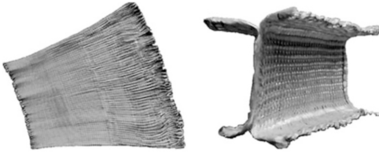
Figure 6.22 Shaping by means of structural variation by adjustment of the stitch length ( left ) and of the binding ( right )
