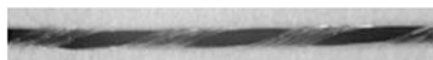
Fig. 4.33 Co-wrapping ply thread, 116 tex fineness, CF filament thread (T300, 67 tex core), wound about with PEEK filament thread (49 tex)
