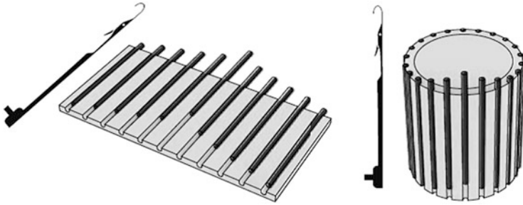
Fig. 6.18 Arrangement of the needle bed on plain flat ( left ) and circular ( right ) knitting machines
