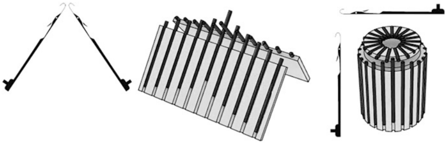
Fig. 6.20 Double jersey knitting process: flat ( left ) and circular ( right ) knitting
