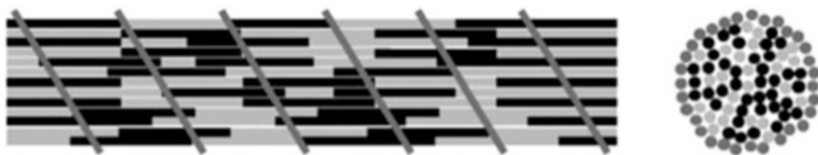
Fig. 4.22 Typical structure of a hybrid core-spun yarn (schematics)
