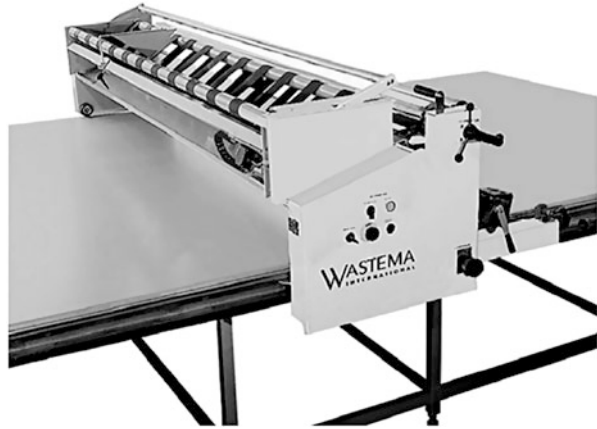
Fig. 12.4 Manual spreading machine with hollow storage of the fabric coil [9] (Source: Wastema International Steinhauser Spezialmaschinen GmbH)
