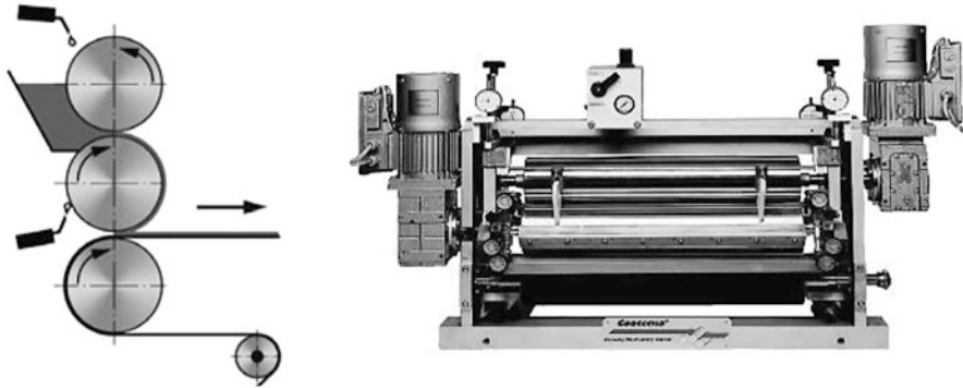
Fig. 13.54 Principle of a reverse roll coater ( left ) and photo of a Coatema plant ( right )
