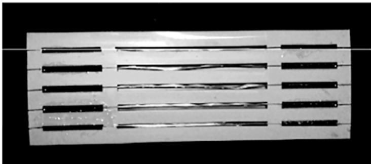
Fig. 14.9 Embedding form for the tensoning of the yarns and application of the load insertion elements
