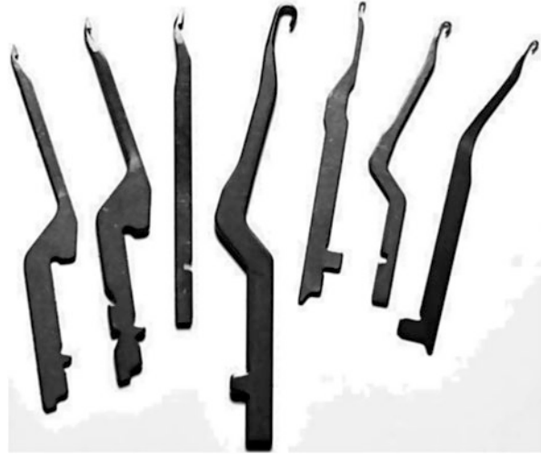
Fig. 7.17 (Piercing) compound needle types (Source: LIBA Maschinenfabrik GmbH)
