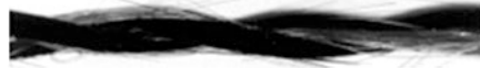
Fig. 4.34 Multifold twisted thread, 232 tex fineness, initial thread made from CF filament thread (T300, 67 tex) and PEEK filament thread (49 tex), pre-twisted thread made from two initial twisted thread
