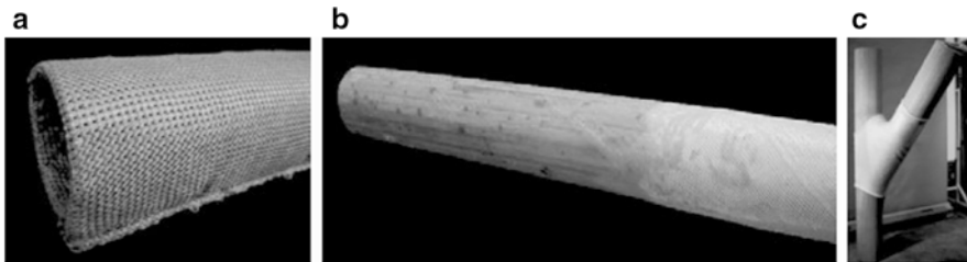
Fig. 6.37 Biaxially reinforced MLG as tubular structures—(a) textile semi-finished product, (b) during application on the surface of a molded wood profile, (c) Y structure as crotch reinforcement
