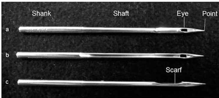
Fig. 12.15 View of a sewing machine needle from three sides: (a) back side with scarf left from need eye, (b) needle with long groove to the guide the need thread to eye, (c) side view with scarf left from needle eye
