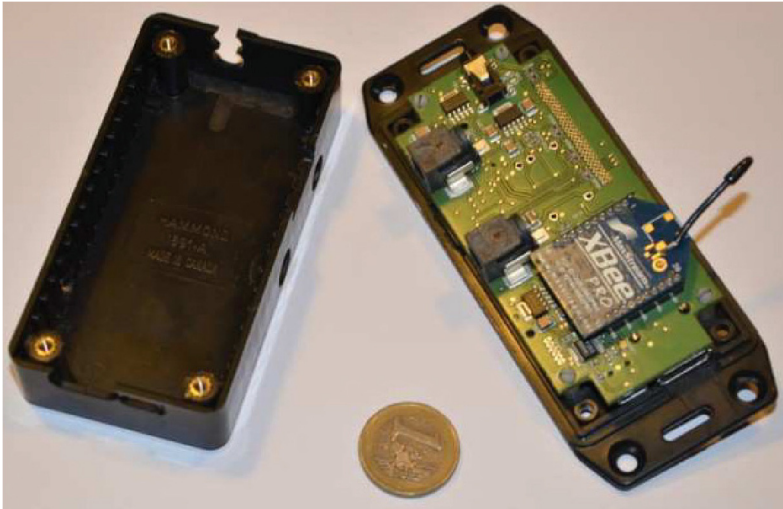
Fig. 3. Airbox – platform based on IGEP development boards, Xbee modem with external antenna is shown attached to the dedicated slot (1 euro coin is used for the comparison of sizes)
