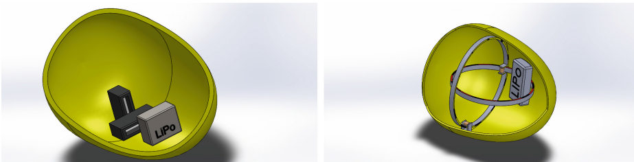
Fig. 6. Mechanisms for changing the center of mass. Left: simplified mechanism based on 2–3 linear motors. Right: advance mechanism allowing to locate the battery mass practically anywhere on the shell.
