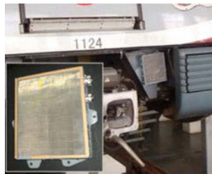
Fig. 5 Onboard transducers of acoustic CAS installed on a vehicle in Shanghai Metro Line 11
