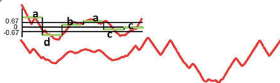
Fig. 2 The SAX word adbacc created from a subsequence of Object1's time series using the sliding window technique
