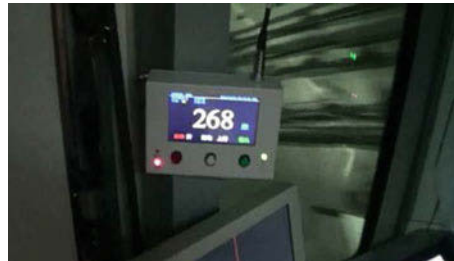
Fig. 6 A snap of the warning display of the acoustic CAS that is switched to the active ranging mode, where the vehicle keeps following a leading one at the speed of 49 \pm 5 km/h in a metro railway tunnel
