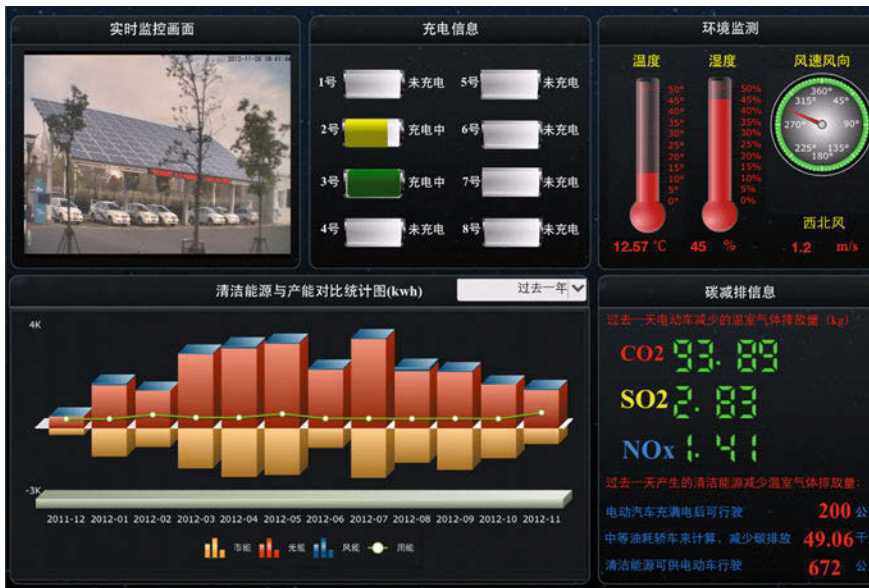
Fig. 7 Page of EVs charging station monitoring
