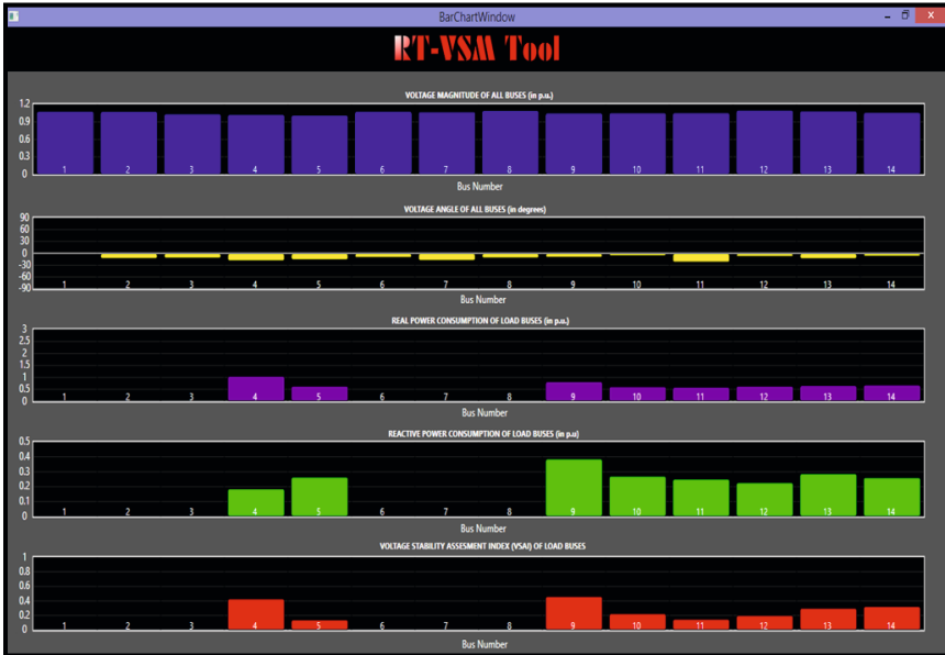
Fig. 16 RT-VSM Tool showing VSAI of all load buses for IEEE 14 bus system
