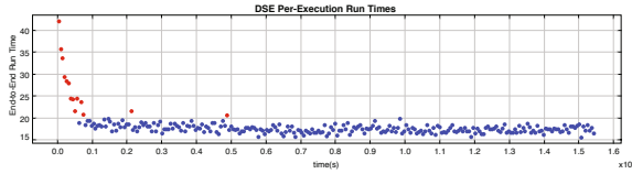
(a) Run-Times of middleware adaptation. [Blue] Executions within deadline, [Red] Executions that missed the deadline
