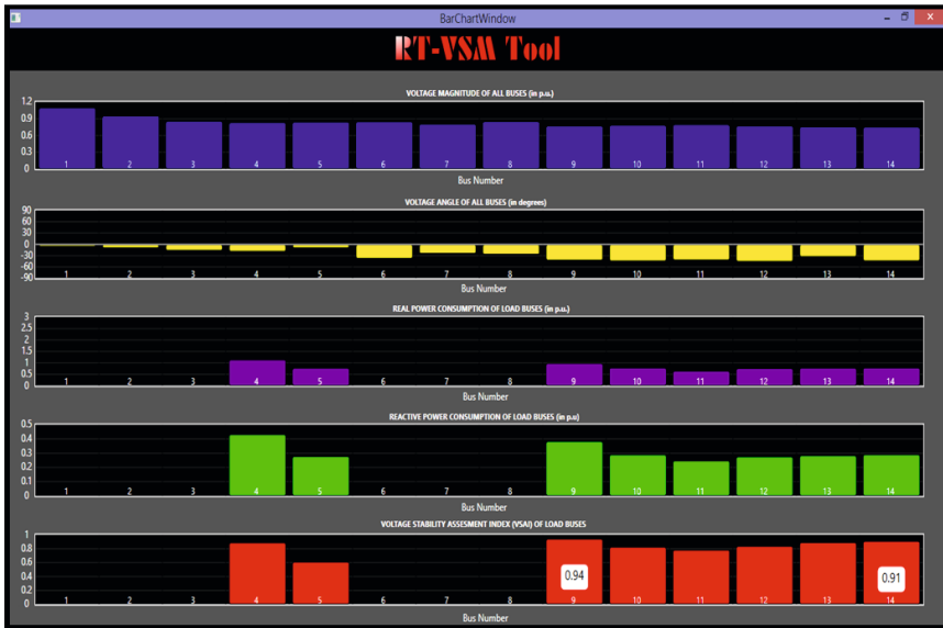
Fig. 17 RT-VSM Tool showing VSAI of all load buses for IEEE 14 bus system following load increase
