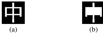
Fig. 4. The effect of filling holes: (a) a Chinese character (b) the effect after filling holes
