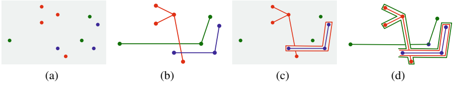
Fig. 4. Steps of the algorithm for the CST problem. (a) An input with n = 10 points and k = 3 . (b) Computing minimum spanning trees. (c) Bounding the tree having the shortest length, and removing red-blue crossings. (d) Merging with the green tree.
