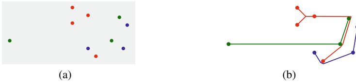
Fig. 3. (a) An input for CST with n = 10 points and k = 3 colors. (b) An optimal solution with minimum ink containing Steiner points.
