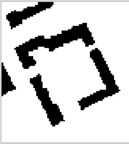
Fig. 5. Building shape after connectivity analysis
