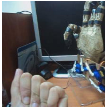
Fig. 10. Real-time manipulation of prosthetic arm using non-amputees
