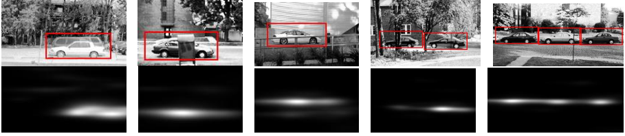
Fig. 4. Examples of detection results. The top row is the location of peaks in energy map of the down row. Objects with some occlusions or multiple instances are detected correctly.
