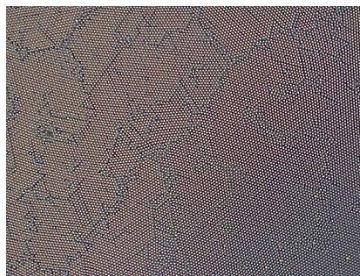
Fig. 3. Microscope image (x100) of HCP silica microspheres ( \varnothing 1.1 \mu\text{m} ) displaying grains separated by fracture lines
