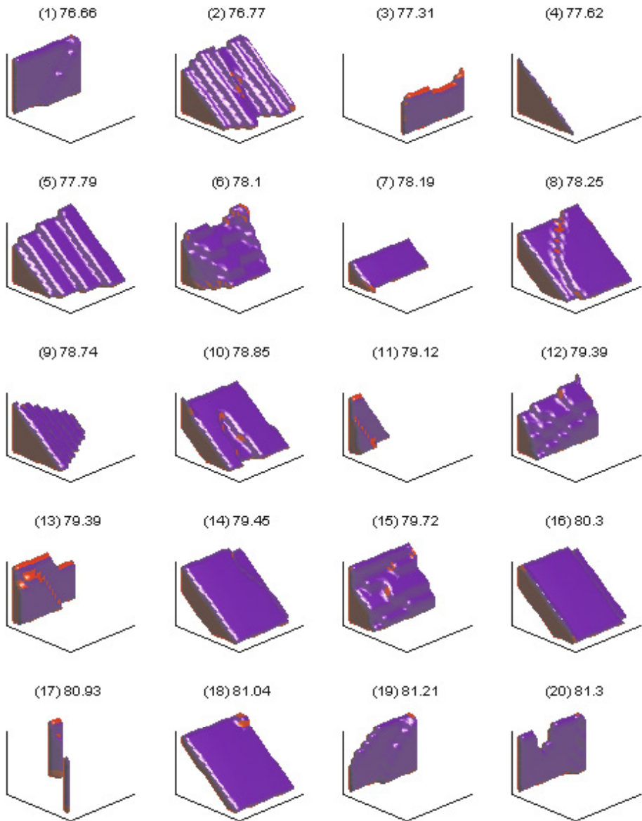
Fig. 3. All final optimised two-material forms with fitness values. Support is red, PV panel material is blue.
