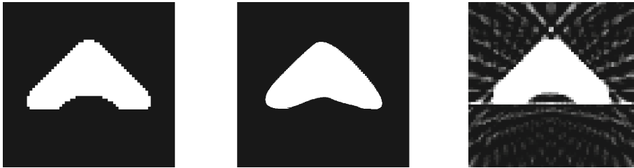
Fig. 7. Left: Original \Omega_2 . Center: NURBS-MCMC reconstruction. Right: FBP reconstruction. Both are using error 0.1%
