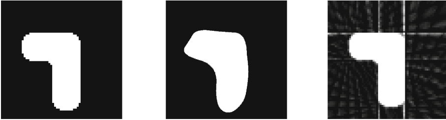
Fig. 6. Left: Original \Omega_1 . Center: NURBS-MCMC reconstruction. Right: FBP reconstruction. Both are using error 0.1%
