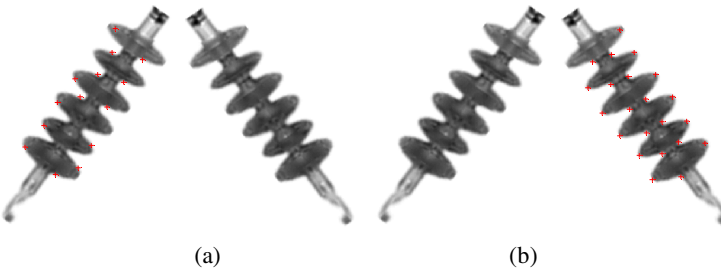
Fig. 10. Candidate points of each connected contour in Im 2. (a) Candidate points of contour 1. (b) Candidate points of contour 2.
