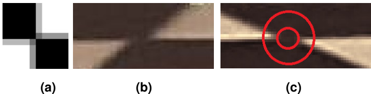
Fig. 5. sampling circle (a) ideal vertex (b) vertex with blurriness(c)sampling circles of different sizes
