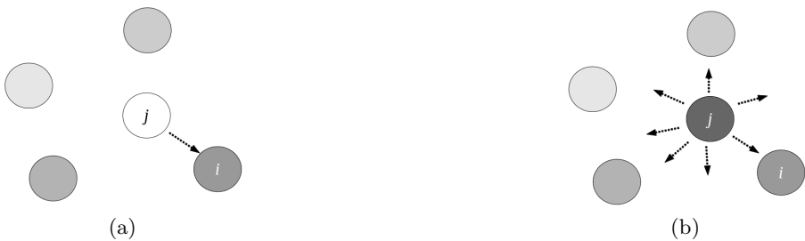
Fig. 1. Firefly movement considering their attractiveness: (a) j moves to i , the most bright firefly close to it; (b) j has more brightness than the most attractive firefly i , so j moves randomly
