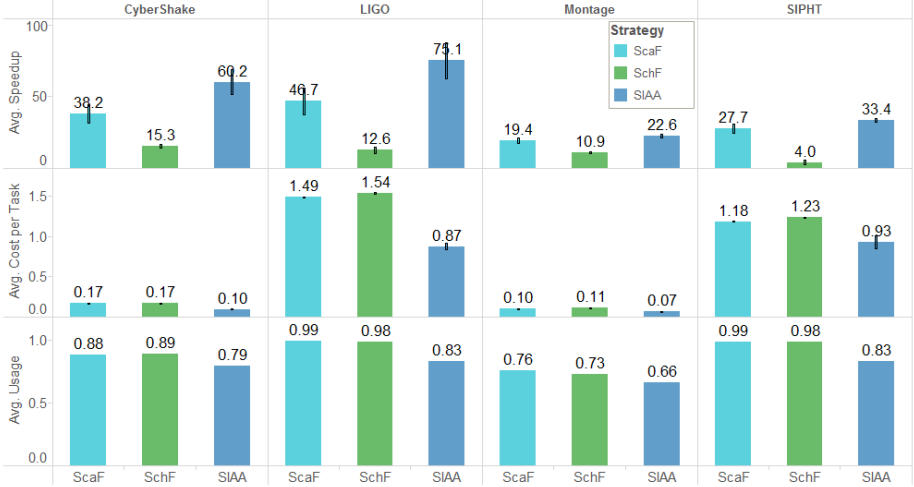
Fig. 3. Performance comparison for each type of workflow. Three autoscaling algorithms are analyzed: (a) Scaling First (ScaF), and (b) Scheduling First (SchF) and (c) SIAA. Algorithms are compared considering speedup, average execution cost per task and efficiency.
