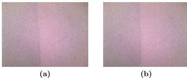
Fig. 5. Consecutive images of the QA3 data set carpet, which are rotated 0.008rad between them. The lack of intensity features make very difficult the use of traditional feature trackers
