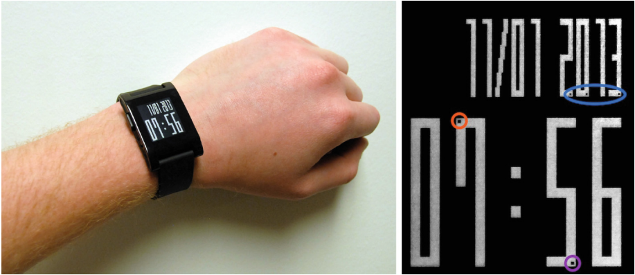
Fig. 3. ConTest Prototype —At a distance ( left ), the application appears to be an innocuous clock face. Closer inspection reveals the question number and answer displays ( right ), encoded in groups of missing pixels (Color figure online).
