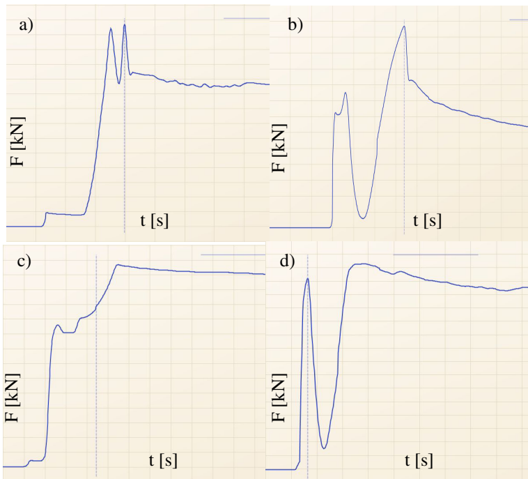
Fig. 2. The slipping curve of the coupling [own study]
