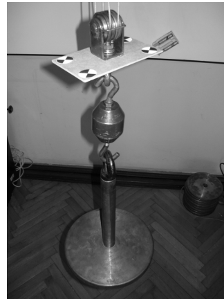
Fig. 2. The hook block with the plate with markers [own study]
