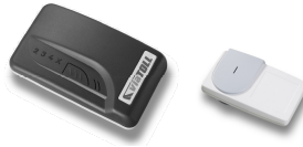
Fig. 1. OBUs used in PTCS for Heavy Vehicles and Light Vehicles [own study]
