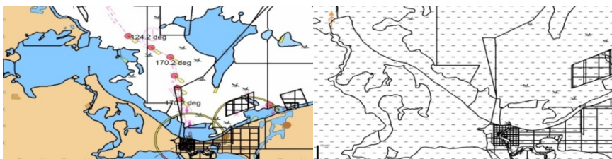
Fig. 1. Electronic navigational chart and its vector representation [9]
