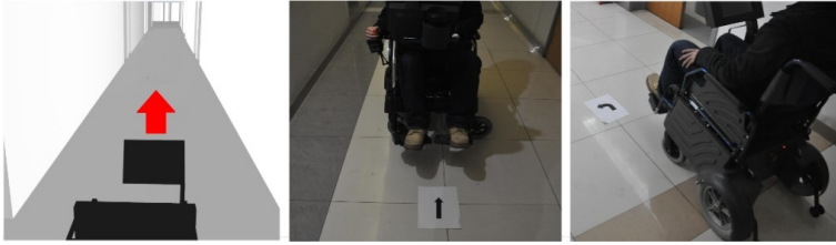
Fig. 8. Three Training Tasks on simulation platform or real electric wheelchair
