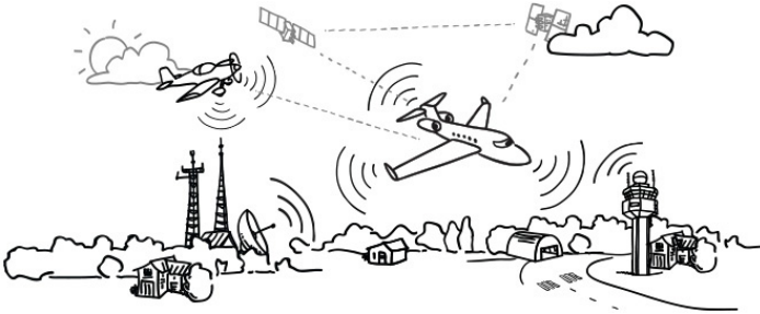
Fig. 14. Overview of the ADS-B system
