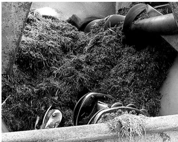
Fig. 1 A mixture of grass and maize silage fed into a biogas fermenter
