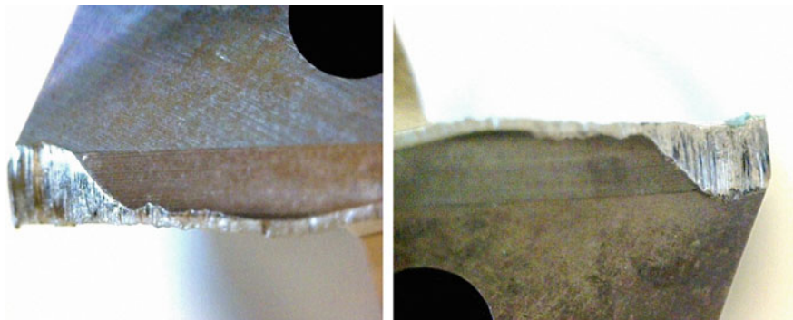
Fig. 1.3 Abrasive wear of the drill corners
