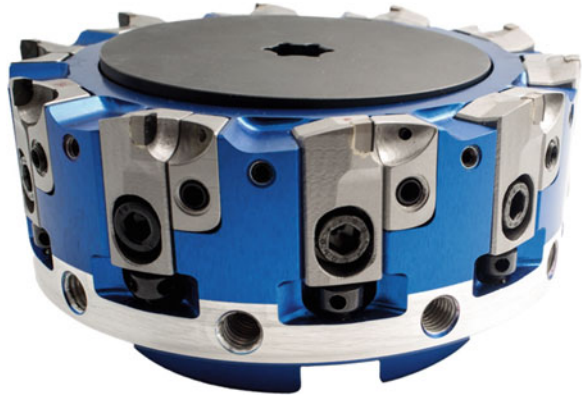
Fig. 1.12 Face milling tool with PCD-tipped cartridges used to represent classification of PCD wear patterns
