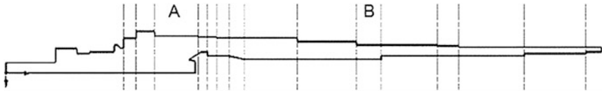
Fig. 7.2 Initial spindle assembly model partitioning and bearing location
