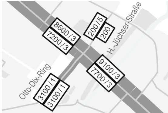
Fig. 1. Part of a traffic volume map (format: daily traffic/percentage of heavy traffic)
