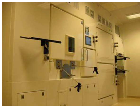
Fig. 7.1 Example of a GMP-clean room for the production of PET radiopharmaceuticals
