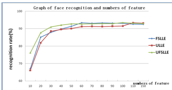
Fig. 1. The average recognition rate of FSLLE, ULLE and UFSLLE changes with characteristic dimension
