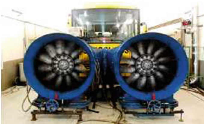
Fig. 21.5 Chassis dynamometer setup at Millbrook
