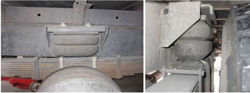
Fig. 4.16 Actual road test vehicle with rubber auxiliary spring
