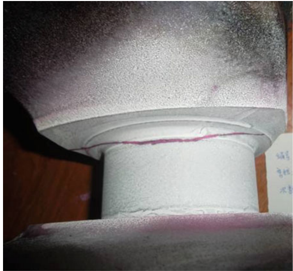
Fig. 12.8 Fatigue failure location of crankshaft
