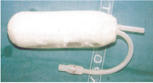
Fig. 2.12 Expanding device constituted of a polyurethane foam body wrapped with an expanding silicone cylinder which may expand under atmospheric pressure
