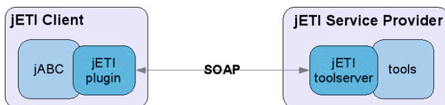
Fig. 8. Schema of Client-Server Interaction Using the ETI Technology
