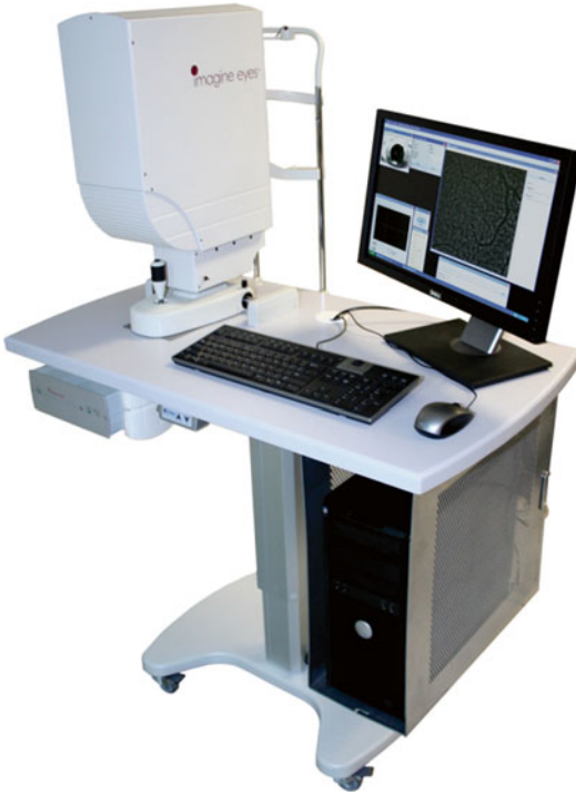
Fig. 7.1 Flood imaging adaptive optics fundus camera developed by Imagine Eyes
