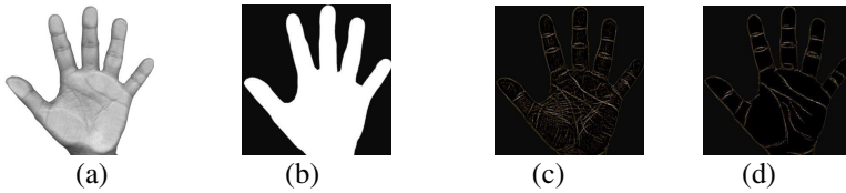
Fig. 2. Original palm vein image, Palm contour segmented using Otsu’s method, Palm Feature obtained using TFSA and Optimized using PGFSR
