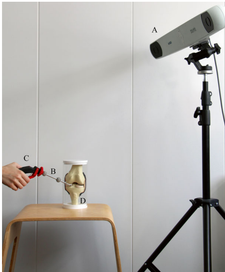
Fig. 13.1 Example of an infrared camera tracking system used in combination with passive reflective markers. (a) Infrared camera. (b) Two markers attached to the shaft of (c) The arthroscopic punch. (d) Anatomic bench model of the knee joint (© GJM Tuijthof, 2014. Reprinted with permission)
