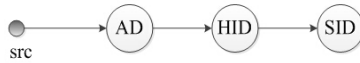
Fig. 4. An simple example of XIA address expressed in the DAG form ( src indicates a virtual source of DAG. AD is a 160-bits number identifying an AD. Similarly, HID and SID are 160-bits identifiers presenting a host or a service).
