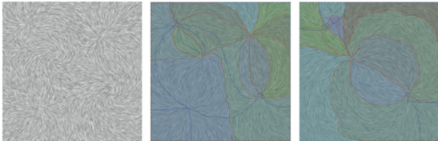
Fig. 4 A two-dimensional vector field ( left ) is decomposed into a rotation free ( middle ), and \pi/2 -rotated divergence-free ( right ) components. These derived fields are segmented with our new approach
