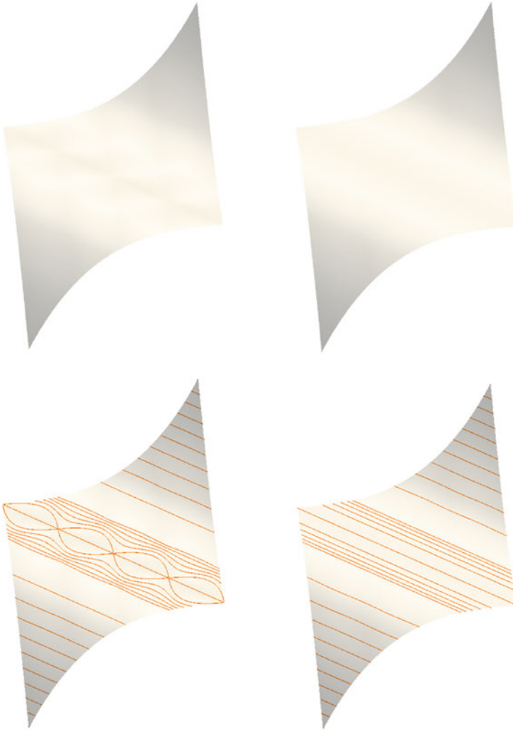
Fig. 9 Interpolation of a grid sampled from an analytical function. The left part shows the result when the exact partial derivatives of the function are used for the interpolant. The isolines on the bottom left clearly indicate critical points. In the right part these critical points are removed by modifying the partial derivatives with our Algorithm 1 (Sect. 3.4)
