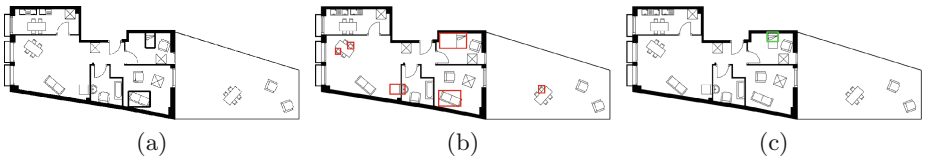
Fig. 10. Results of detecting bed , here the single instance of bed is correctly detected, note that in this case the instance is also attached with thin black pixel, (b) Results of spotting bed by the previous version of the method [3], (c) Results of spotting bed by Dutta et al. [7].
