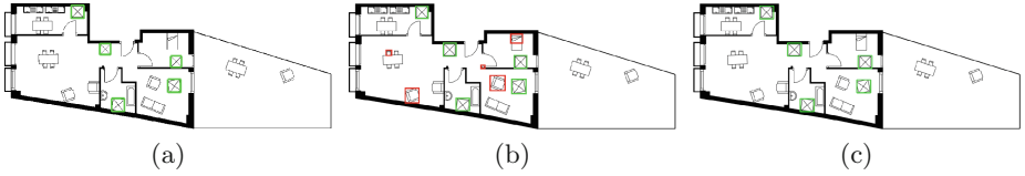
Fig. 8. Results of detecting table1 , note that all the instances of the symbol table1 are correctly detected even the one which is connected with thick black pixels, (b) Results of spotting table1 by the previous version of the method [3], (c) Results of spotting table1 by Dutta et al. [7].
