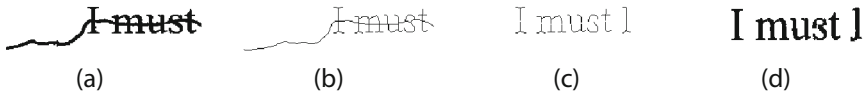
Fig. 5. (a) Segmented object from original image in Fig. 3. (b) Skeletonized version of the object in (a). (c) Line removal. (d) Dilated version of (c) assuming as limit the corresponding areas in image (a).
