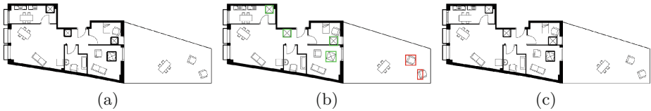
Fig. 6. Results of detecting table1 , note that all the instances of the symbol table1 are correctly detected even the ones attached with the walls. In reality these walls are thin and hence less distorted during the vectorization, (b) Results of spotting table1 by the previous version of the method [3], (c) Results of spotting table1 by Dutta et al. [7].
