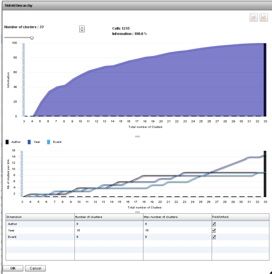
Fig. 3. Choosing the wanted granularity for visualizing the grid is available through the “Unfold Hierarchy” functionality. The user can control either the number of parts of the dimensions or the grid quality (w.r.t. to the optimal grid) by optimal merging or per-dimension customized non-optimal merging.
