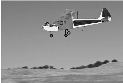
Fig. 3. SIG Rascal 110 research aircraft operated by the Naval Postgraduate School for time-critical cooperative missions. Onboard avionics include the Piccolo Plus autopilot, two PC-104 industrial embedded computers, and a wireless MANET link for air-to-air and air-to-ground communications. (See [36] for a detailed description of these avionics.)
