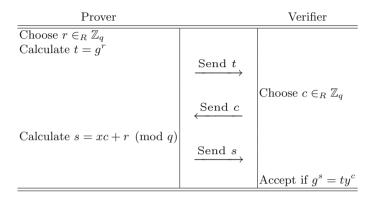
Fig. 1. Schnorr protocol for proving knowledge of a discrete logarithm.
