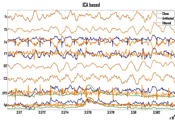
Fig. 5. The ICA-based method. Most of the electrode signals correctly remain intact but the artifact related electrodes, as well as the ones containing some sort of components that fulfilled the removal criteria, have lost the texture of the reference signal.
