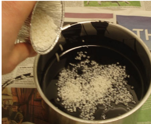
Fig. 10.8 Sasobit addition to binder in laboratory
