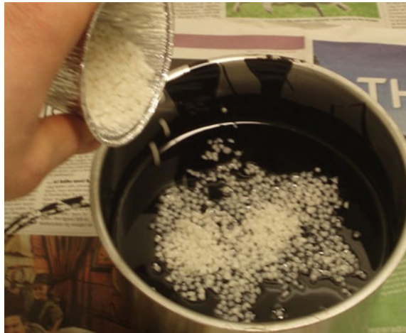
Fig. 10.8 Sasobit addition to binder in laboratory
