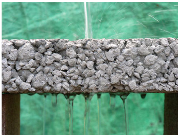
Fig. 16.7 Pervious concrete (Source Gaia engineering)
