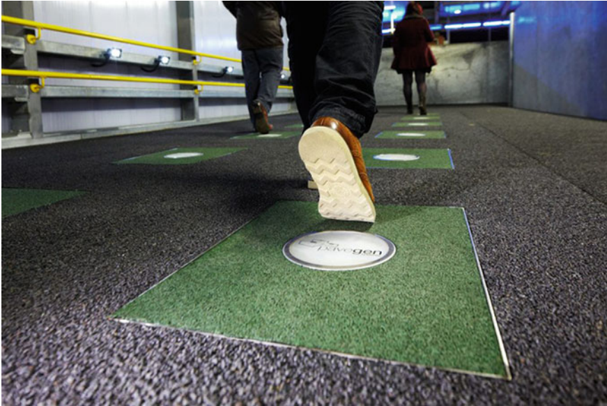
Fig. 18.13 Pavegen: kinetic energy generation from footsteps (Pavegen 2012)
