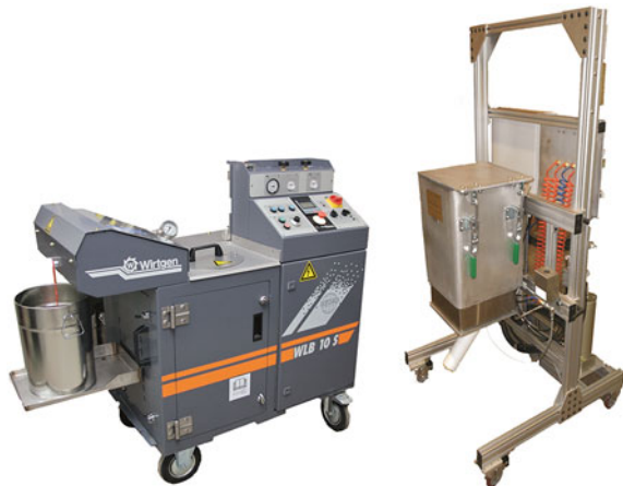
Fig. 10.10 Wirtgen WLB 10 S ( left ) and Pavement Technology's The Foamer ( right ) laboratory foaming units
