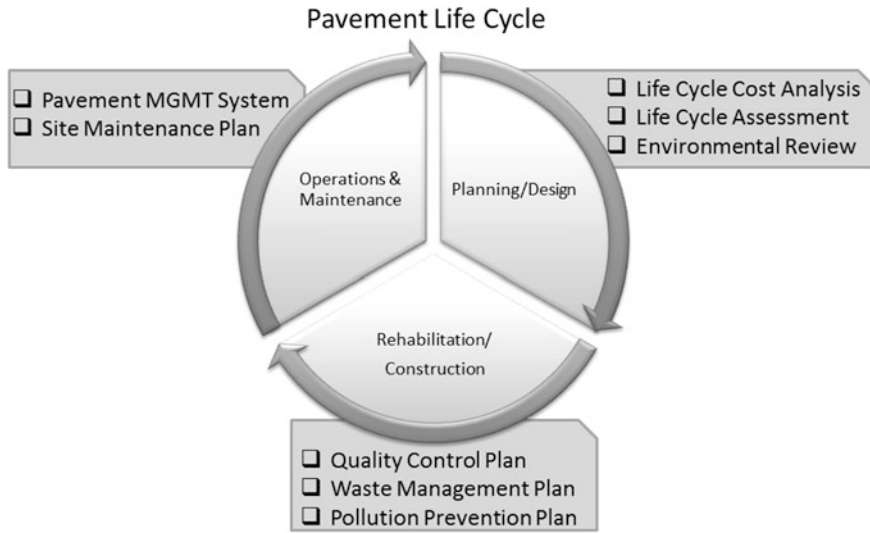
Fig. 12.1 Fundamental practices for pavement life cycle sustainability
