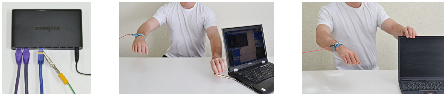
(a) Measuring shield potential at the far side of an Ethernet cable (probed at the Ethernet switch). (b) Non-adaptive “human touch” attack through a metal pen touching the heatsink fins. The wristband is connected to the probe wire. (c) Adaptive “human touch” attack by bare hand. The wristband is connected to the probe wire.
