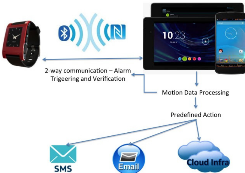
Fig. 1. Architecture of the proposed fall detection application
