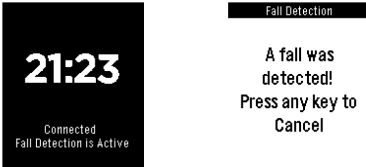
Fig. 3. Screenshots of the Pebble Smart watch Application in case of an idle active connection and in case of a detected fall
