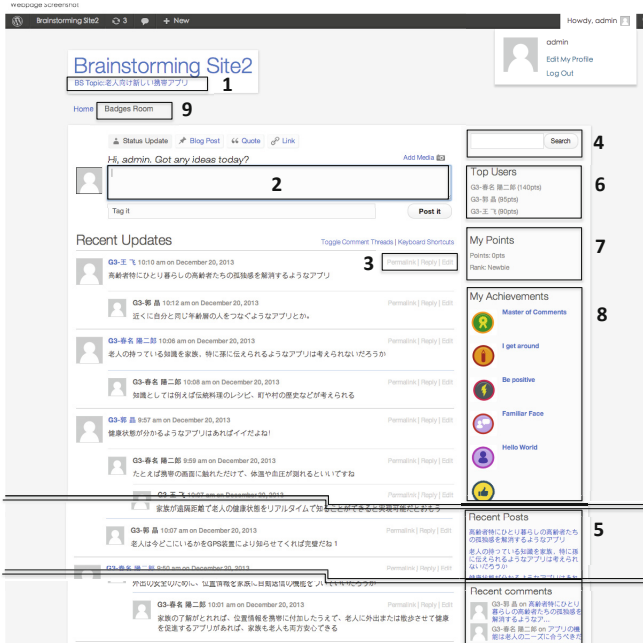
Fig. 1. Interface screen of the electronic brainstorming system with the following gamification elements indicated: Area 1, brainstorming theme; Area 2, input idea; Area 3, reply to an existing idea; Area 4, text-search function; Area 5, current ideas; Area 6, leaderboard; Area 7, user level and score; Area 8, badge list; Area 9, information about all badges
