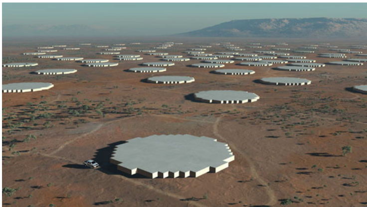
Fig. 1.8 SKA dense aperture array station made up of 3 m x 3 m “tiles” for medium frequencies of about 500 MHz–1 GHz. Graphics: Swinburne Astronomy Productions and SPO
