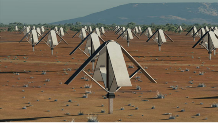
Fig. 1.6 SKA sparse aperture array station of dipole elements for low frequencies of about 50–350 MHz. Graphics: Swinburne Astronomy Productions and SKA Project Office (SPO)
