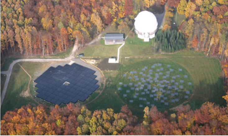
Fig. 1.5 International LOFAR station near Tautenburg/Germany. Left: dense array of dipole “tiles” for frequencies of 110–240 MHz, right: sparse dipole array for 10–80 MHz; top: optical Schmidt telescope (copyright: Michael Pluto, Thüringer Landessternwarte)
