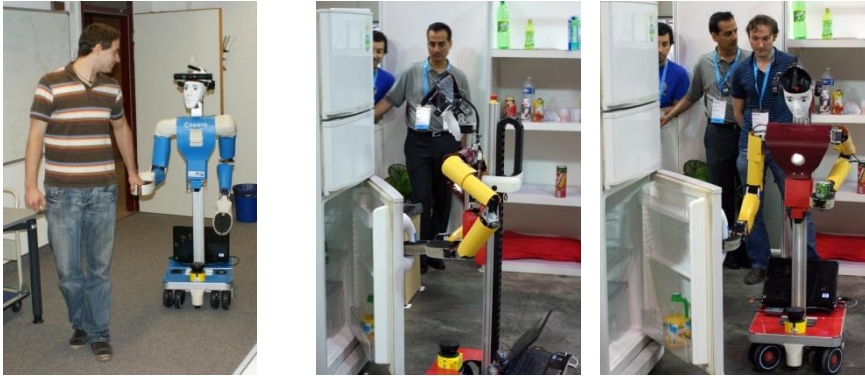
Fig. 7.3 Left: A person guides Cosero at its hand. Right: Dynamaid opens and closes a refrigerator using compliant control at RoboCup 2010 in Singapore.
